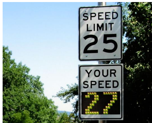
Figure 6.12: Radar speed check sign
