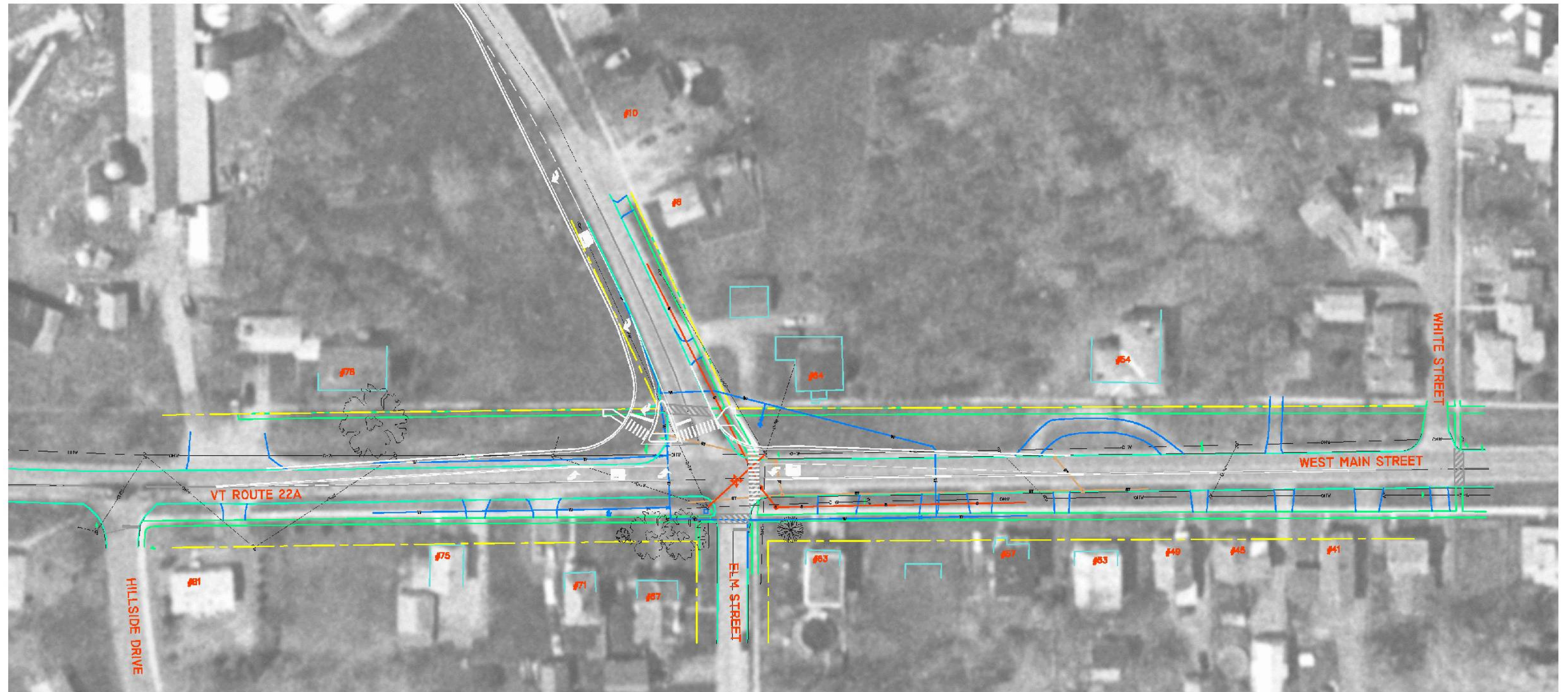
Figure 11 Alternative C2 – Two-Way Stop Control w/ Route 22A and Panton Road Widening
