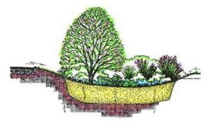
Bioretention areas are depressions constructed to treat stormwater as it flows through vegetation and soil before entering the storm drainage system. Parking lot islands are good candidate sites for bioretention.
