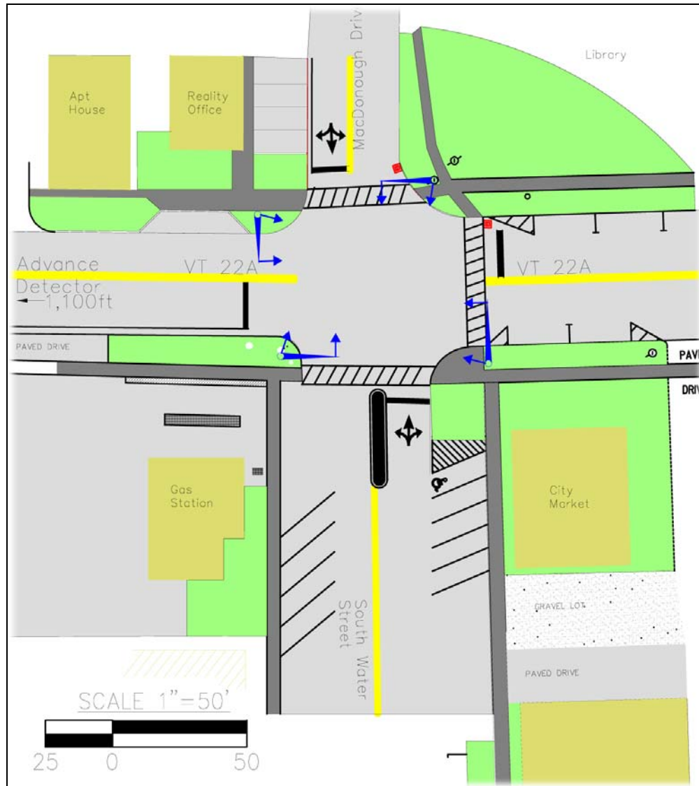
Figure 25: Alternative 1 Traffic Signal and Median – Conceptual Design
